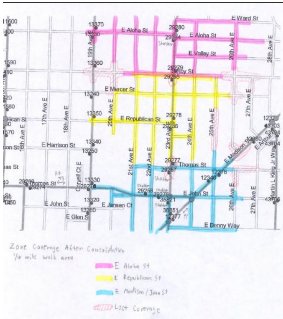
Figure 5: Example of a bus stop coverage sketch, superimposed on a GIS-generated street network map. Small circles are bus stops, with bus zone ID number shown, larger circles are traffic signals. The three highlight colors represent the coverage area from the three pairs of bus stops that would remain. The red crosshatch shows the area that would no longer be within a ¼ mile walk of a bus stop, if the two pairs of bus stops, circled in red, were removed. (Note that neither of these bus stops were actually closed, due to customer opposition)
